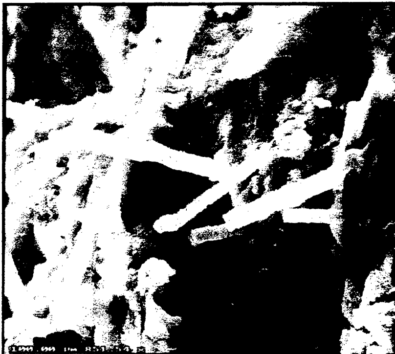
Figure 2. Scanning Electron Micrograph of dried, natural floc, showing backbone and aluminosilicate tubules (approximately 40 \mu\text{m} long)
